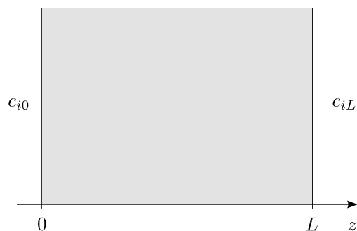
Figure 2.1: A membrane separating two reservoirs of constant concentration c_{i0} and c_{iL} , respectively. The direction of diffusive transport is along the z direction, and L denotes the thickness of the membrane.
