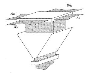
Figure 2: The multiplier for  $Z_R$  or  $Z_I$ . The complete complex multiplier consists of two of these. Partial inner product generator at top, adder tree in the middle and fast carry-lookahead adder at the bottom.
