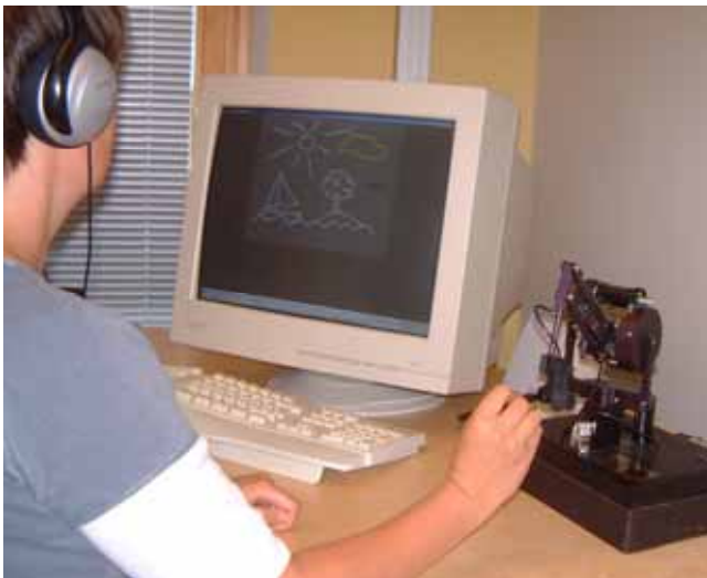
Figure 1 A person using a haptic desktop device (the PHANToM) for editing a digital hand drawing
