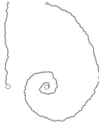
Fig. 15 Trails with 40^\circ angle deviation. One trail using the random interval approach with a 10^\circ angle interval (left) and one worst-case trail for 150^\circ (right)
