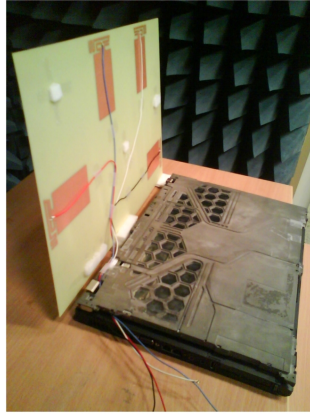
Figure 5: Photo of the laptop equipped with four antennas.
