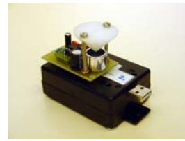
Fig. 2. Stationary sensor network nodes with ultrasound receiver circuit. The node is packaged in a plastic box to reduce wear.
