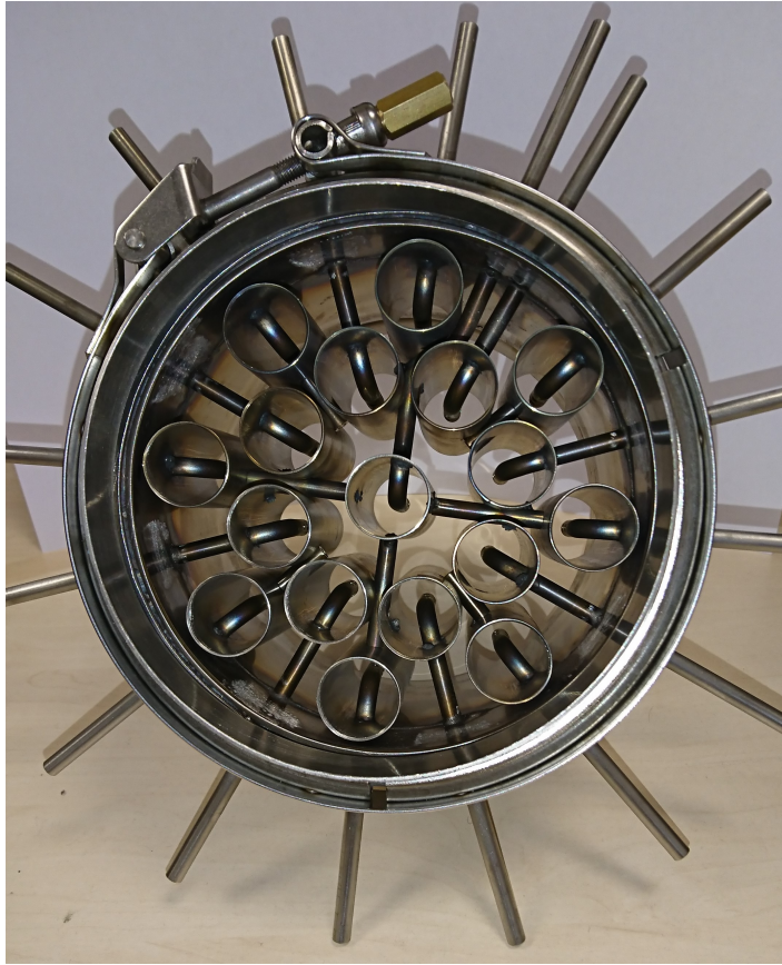
Figure 7.2: The exhaust probe unit included the 17 different locations for individual exhaust probe measurement.
