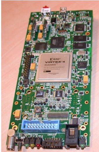
Figure 5: View of the prototype board for HDR system. (Courtesy: CEA/LETI, Grenoble)
