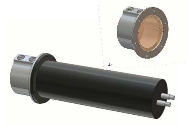
Figure 2: The NE-213 reference detector. Top: a detail of the cylinder “cup”. The screws on top allow for the filling or draining of the liquid cylinder. A borosilicate-glass window (light brown) serves as the optical boundary. See text for details. Bottom: The black cylinder to the right is the magnetically shielded 3 inch ET Enterprises 9821KB photomultiplier-tube assembly. The gray cylinder to the left is the “cup”. (For interpretation of the references to color in this figure caption, the reader is referred to the web version of this article.)
