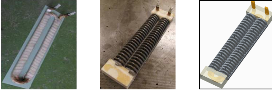
Figure 22: GreenHeat inductor: Left: Naked coil. Center: Finished inductor. Right: CAD model [49].
