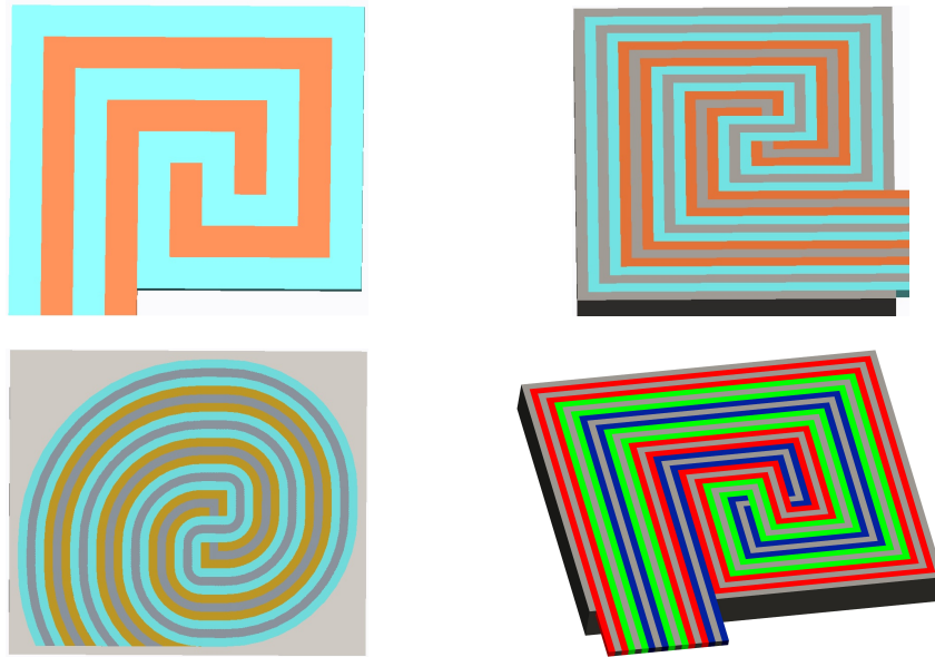
Figure 74: Different conceptual coil designs in order to eliminate coil ends.
