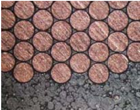
Figure 21: Coil surrounded by a molded flux concentrator made of SM 2 C material [50].
