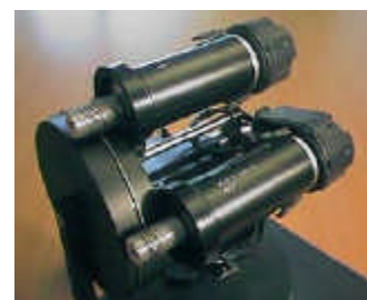
Fig.2. The PHANToM and a close-up of two motors
