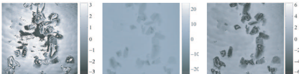
Figure 3: Amplitude images of lactose crystals mounted in a liquid with n_m = 1.570 . The Becke lines move out from the crystals into the liquid as the image plane is shifted in the direction of the illuminated wave, i.e. , towards the sensor from -100 \mu\text{m} to 100 \mu\text{m} .
