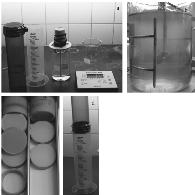
Figure 10 a) Transparent Plexiglas® cylinder with filter element installed, 1000 ml measuring cylinder, Kemira Flocculator 2000 b) variable speed flocculator c) cylinder filter elements d) cylinder filter element mounted on the Plexiglas® cylinder with a flexible pipe coupling.
