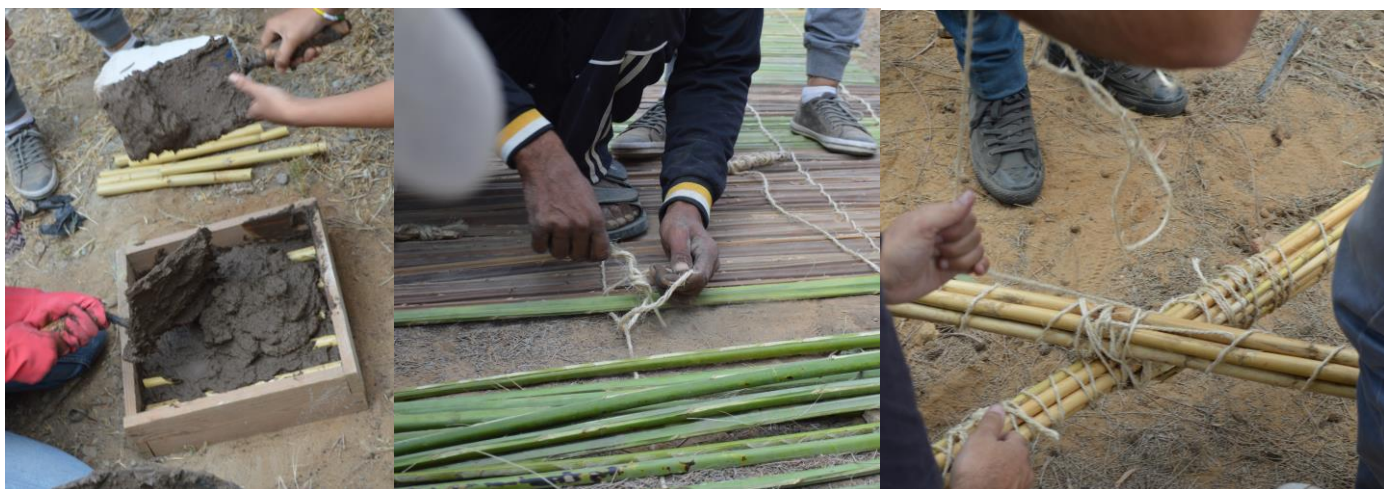
Fig (11) Testing different applications for using reeds in walls and roof construction. Photos Credits; Insaf Ben Othman
