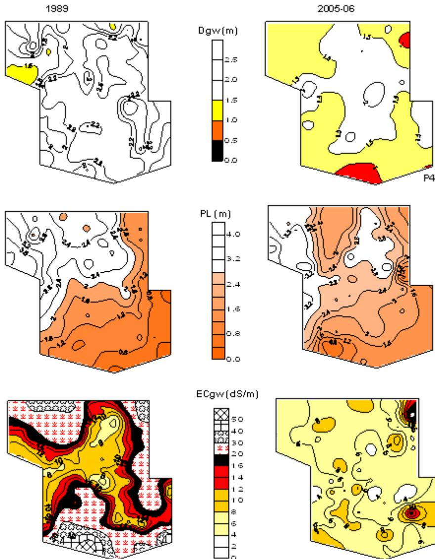
**Fig. 4.** Spatial distribution of groundwater properties before irrigation (October 1989) and after over 17 years of soil reclamation (2005-2006). Groundwater depth ( $D_{gw}$ , m), piezometric level ( $PL$ , m) and electrical conductivity ( $EC_{gw}$ ,  $\text{dS}\cdot\text{m}^{-1}$ ).
