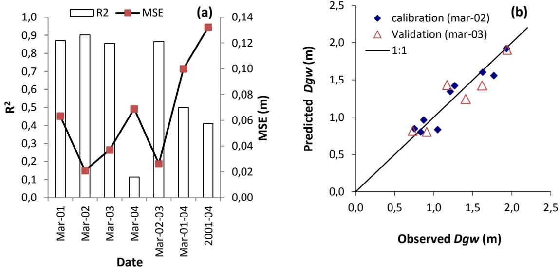
Fig. 4 (a) The performance of the best SLR model to predict  $D_{gw}$  from  $EM_v$  at various time measurements (b) Observed and predicted  $D_{gw}$  (m) for calibration (March 2002) and validation (March 2003) subset.
