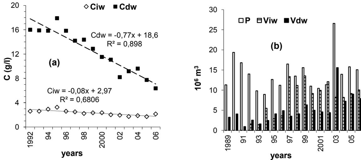
**Figure 20.** Annual variation of total dissolved salts and volume of irrigation water ( $C_{iw}$ ,  $g.l^{-1}$ ;  $V_{iw}$ ,  $10^6 m^3$ ), total dissolved salts and volume of drainage water ( $C_{dw}$ ,  $g.l^{-1}$ ;  $V_{dw}$ ,  $10^6 m^3$ ) and precipitation ( $P$ ,  $10^6 m^3$ ).
