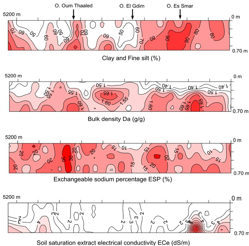
**Figure 4.** Impact of the old arms of Medjerda River (O. Oum Thaaled, O. El Gdir and O. Es Smar) on spatial variation of soil salinity, exchangeable sodium percentage and bulk density at 0-0.75 m soil depth at the transect T1.
