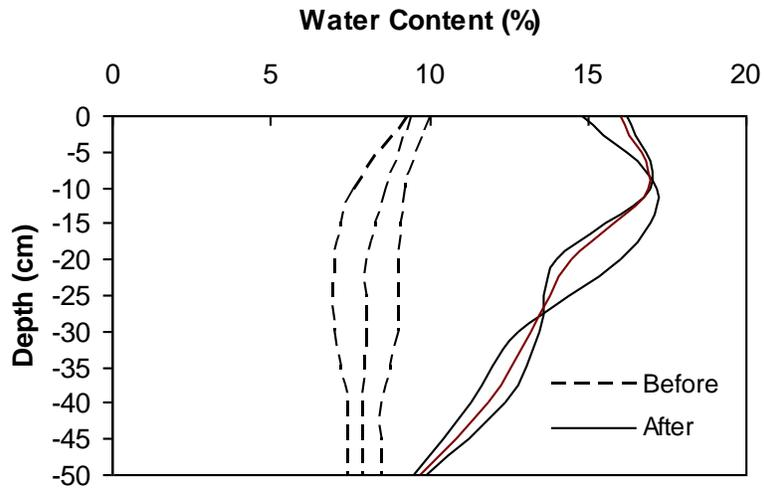
Fig. 3 Soil water content before and after infiltration
