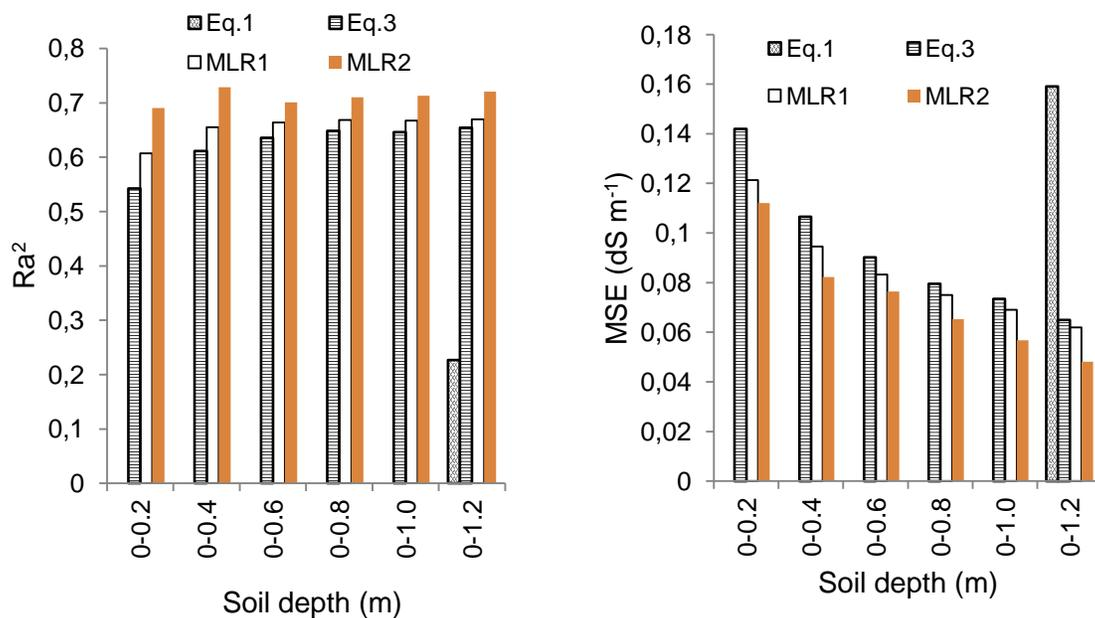
Fig. 2 Adjusted  $R^2$  ( $Ra^2$ ) and mean square error (MSE) of predicting  $\ln ECe$  observed at various soil depths and seasons (12 campaigns from 2001 to 2004) with various models (equations (1) and (3), and MLR). MLR1: EM variables and plot coordinate as predictors; MLR2: same inputs than MLR1 plus groundwater properties.
