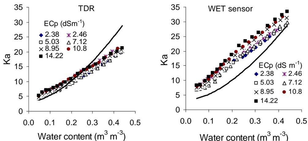
**Fig. 2** The soil dielectric constant ( $K_a$ ) measured with TDR and WET sensor vs water content ( $\theta$ ) for each pore water electrical conductivity ( $EC_p$ ). The solid line represents the Topp *et al.* (1980) equation.
