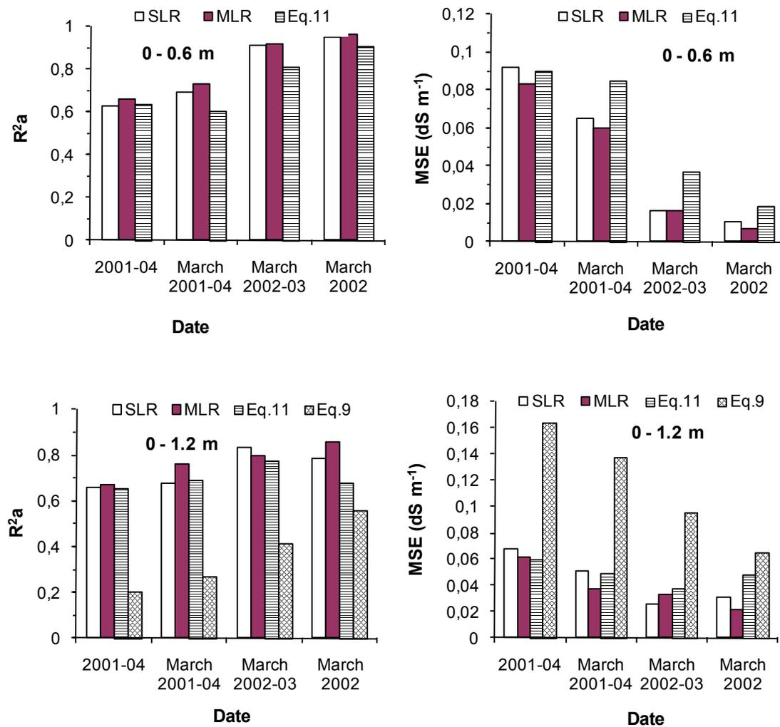
**Figure 12.** The  $R^2_a$  and MSE of predicting  $\text{Ln}EC_e$  at various soil depths (0-0.6, 0-1.2 m) and date of measurement using various models (Eqn. (9), Eqn. (11), best SLR and MLR models). For MLR, EM and plot coordinate variables were used as predictors.
