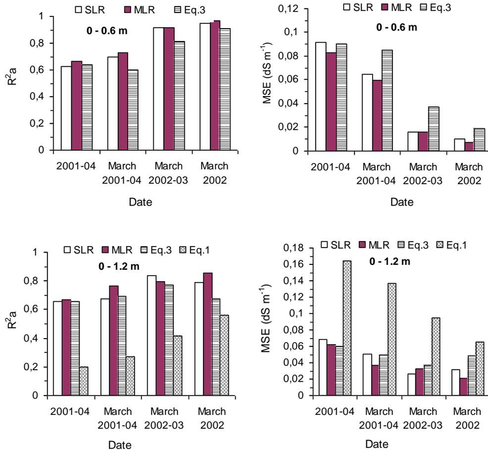
Fig. 3 The  $R_a^2$  and MSE of predicting  $\ln EC_e$  at various soil depths and date of measurement using various models (equations (1) and (3), best SLR and MLR models). For MLR, EM and plot coordinate variables were used as predictors.
