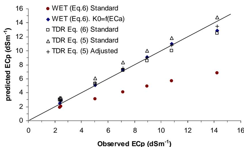
Fig. 6 The pore electrical conductivity ( $EC_p$ ) observed and predicted by Hilhorst (2000) (equation (6)) and Malicki & Walczak (1999) (equation (5)) with the WET sensor and TDR. The standard and adjusted parameters of both models were used to predict  $EC_p$ .
