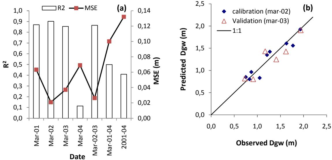
**Figure 13.** (a) The performance of the best SLR model to predict Dgw from EMv at various time measurements. (b) Observed and predicted Dgw (m) for calibration (March 2002) and validation (March 2003) subset.
