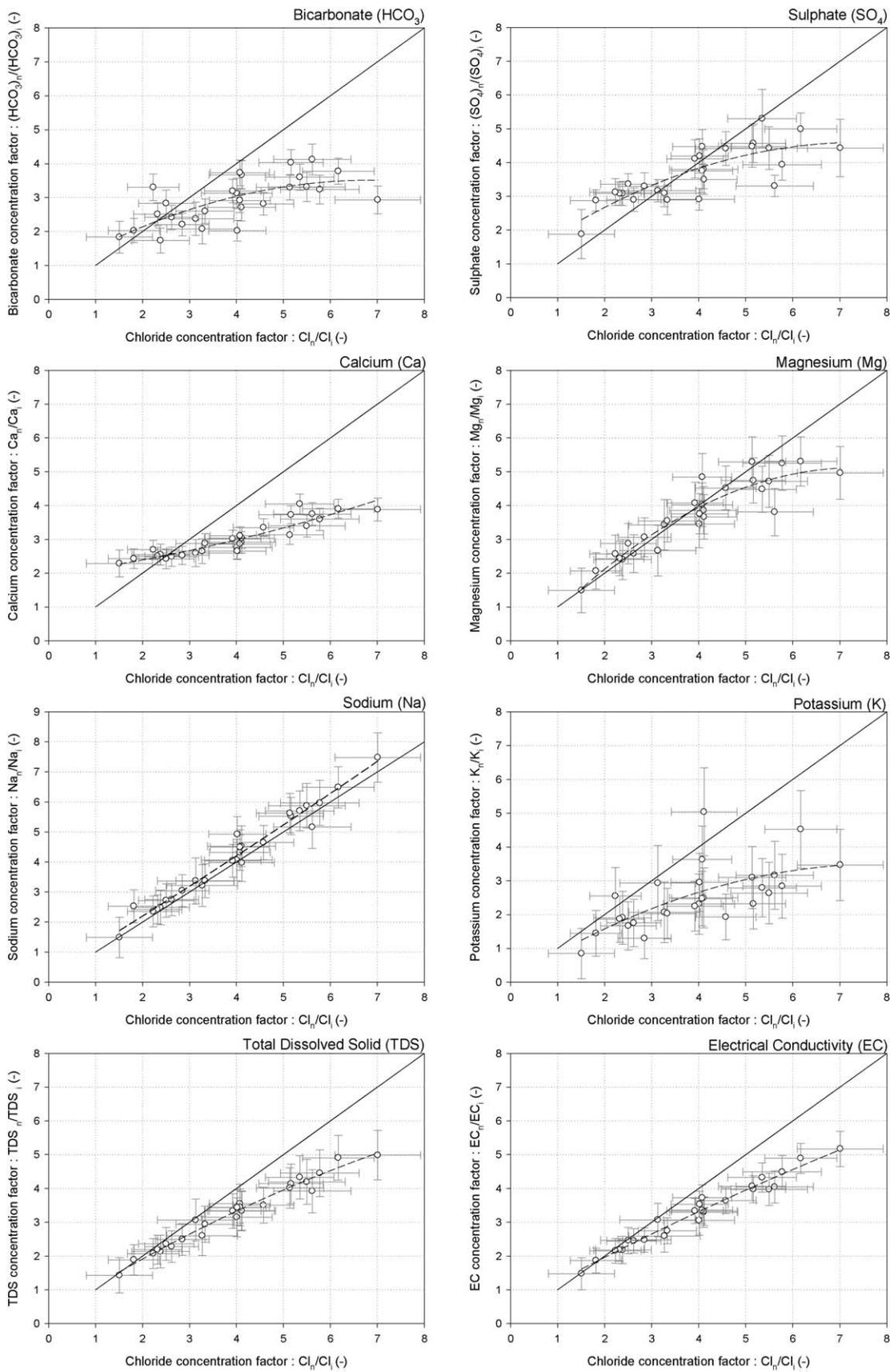
**Fig. 3.** Concentration diagrams of bicarbonate, sulphate, calcium, magnesium, sodium, potassium, the total dissolved solids (TDS) and the electrical conductivity (EC) with respect to chloride in groundwater. All concentrations are expressed as concentration factor with respect to the irrigation water (Eq. (3)).
