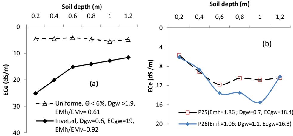
**Figure 11.** Impact of soil water content ( $\theta$ ), groundwater table depth ( $D_{gw}$ , m) and salinity ( $EC_{gw}$ ,  $dS\ m^{-1}$ ) on soil salinity profile ( $EC_e$ ) and EM38 reading (reading at horizontal (EMh) and vertical (EMv) dipole orientation).
