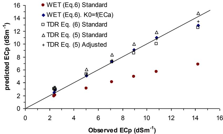
**Figure 10.** The pore electrical conductivity ( $EC_p$ ) observed and predicted by the Hilhorst (2000) (Eqn.(6)) and the Malicki and Walczak (1999) (Eqn. (5)) with the WET sensor and TDR. The standard and adjusted parameters of both models were used to predict  $EC_p$ .
