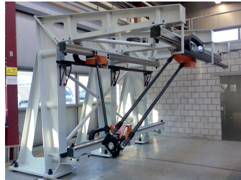
Fig. 1. Full size Gantry-Tau prototype (SMERobot™project)
