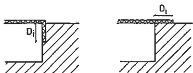
Figure 12.8. Vertical versus horizontal insulation of the upper side of the store.
