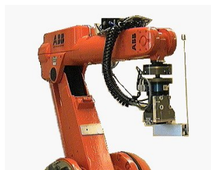
Figure 3: An inverted pendulum actuated by an industrial robot.
