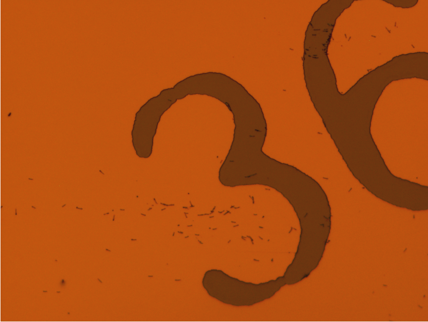
Figure 3.2: Optical microscopy image of nanowires transferred to substrate for optical measurements. The nanowires are about 4 \mu\text{m} long and the substrate is a silicon wafer with patterned gold layer.
