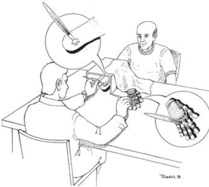
Figure 6.3: Experimental setup. Cyberhand prosthesis in full view and hidden residual limb being stimulated with a brush. Reprinted with permission from Informa Healthcare.
