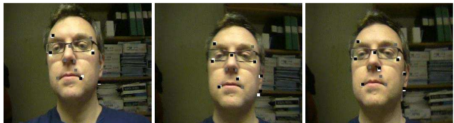
Figure 9.3: Three out of 100 frames used for testing. For measured points (in white) the fitted model points are shown in black. For missing data the fitted model points are shown in gray.
