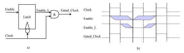
Figure 3: a) Clock gate and b) Timing diagram
