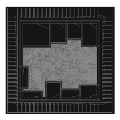
Figure 6: Chip plot of the FFT processor.
