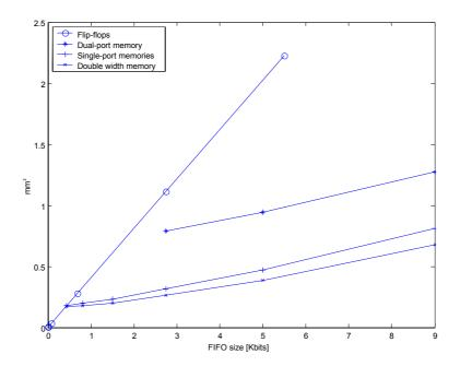
**Figure 5**: Area versus FIFO size for different implementations.
