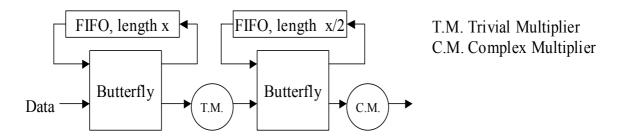
**Figure 1**: A radix  $2^2$  stage.  $x = 2^{2*stage-1}$
