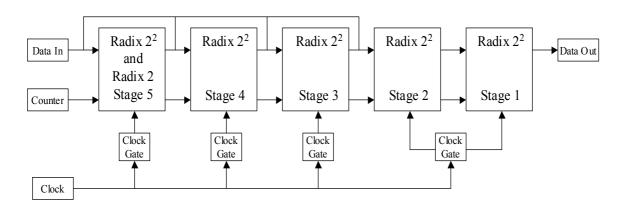
Figure 2: Architecture of the FFT processor.
