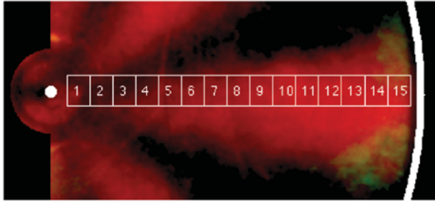
Figure 6. Visualization of the binning zones used for the spectral evaluation of the formaldehyde/PAH LIF along the jet axis.
