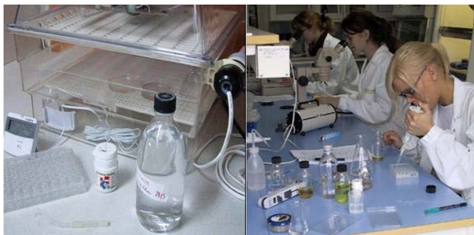
Figure 3. Equipment for hatching the Artemia larvae (left) and procedure for preparing the samples and scoring the results in the acute toxicity test (right).
