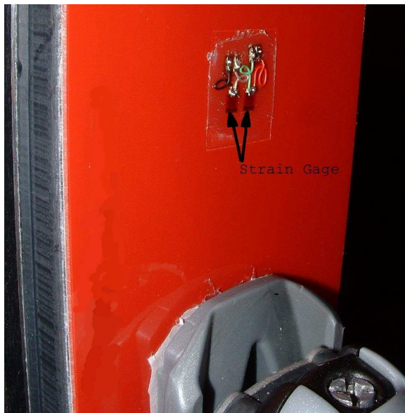
Fig. 2. The strain gages mounted on the ski.
