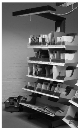
Figure 1. The sorting rack. The top shelf should be at shoulder height for the postal workers. The bottom shelf is mainly used for storage.
