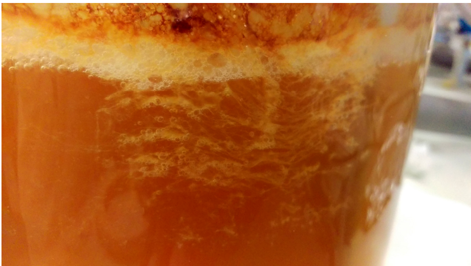
Figure 8 Biofilm formation during co-cultivation of C. saccharolyticus G5 and C. owensensis CO80 cultivated on wheat straw hydrolysate
