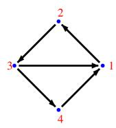
Fig. 1. The graph reflects the interconnection structure of the dynamics between four systems. The arrow from node 1 to node 2 indicates that system 1 affects the dynamics of system 2 directly.
