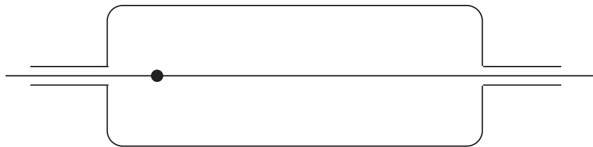
Figure 6.5: The metallic sphere on the symmetry axis of an axially symmetric cavity. The frequency shift of the mode number n is proportional to the square of the electric field at the position of the sphere of the same mode.
