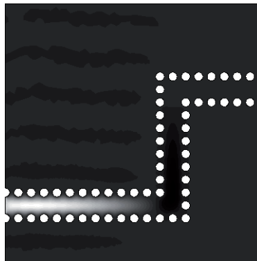
Figure 5.25: The SIW at 30 GHz. No modes are propagating since the frequency is below the cut-off frequency for the fundamental mode.
