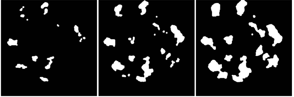
Figure 3.6: Sample images used in the determination of combustion propagation speed. Combustion regions are shown in white. The images are sequential from left to right with a timestep of 32.26 \mu\text{s} .
