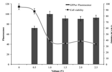
**Fig. 5** Voltage effects on the extraction procedure of the reporter protein GFPuv using a 10 mM citrate buffer containing 10 mM NaCl, 30 mM glucose, pH 5.8. GFP fluorescence of the supernatants and cell viabilities are presented on the y-axis. The error bars indicate standard deviations based on three independent extraction tests and five viability determinations.
