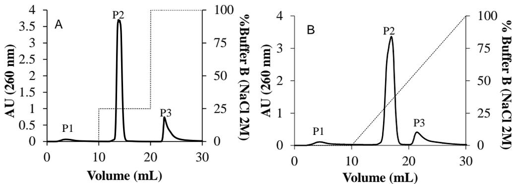
**Figure 2 - Isolation of PCR products using *Capto Adhere*. A – Chromatogram for PCR product purification using a step gradient with 25% Buffer B. B – Chromatogram for PCR product purification using a linear gradient approach until 100% buffer B was reached. The sample applied was a PCR product of 272 bp; Primers used: pET upstream, DuetDOWN1.**
