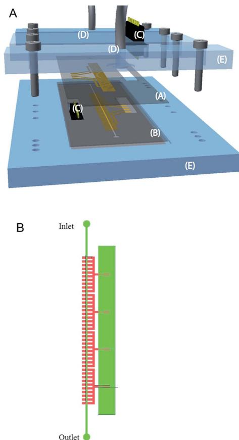
**Fig. 2** (A) – Schematic drawing of the electropermeabilization setup. The exploded view shows the top electrode layer (A), and the middle channel with bottom electrode array (B). Spring loaded connectors are pressed against the contact pads of bottom and top electrodes (C). The fluidic connection (D) is sealed via o-rings (not shown). (E) PMMA holder. (B) – Two-dimensional design of the bottom layer of the chip; red represents the electrode array and green the chip structure and channel.
