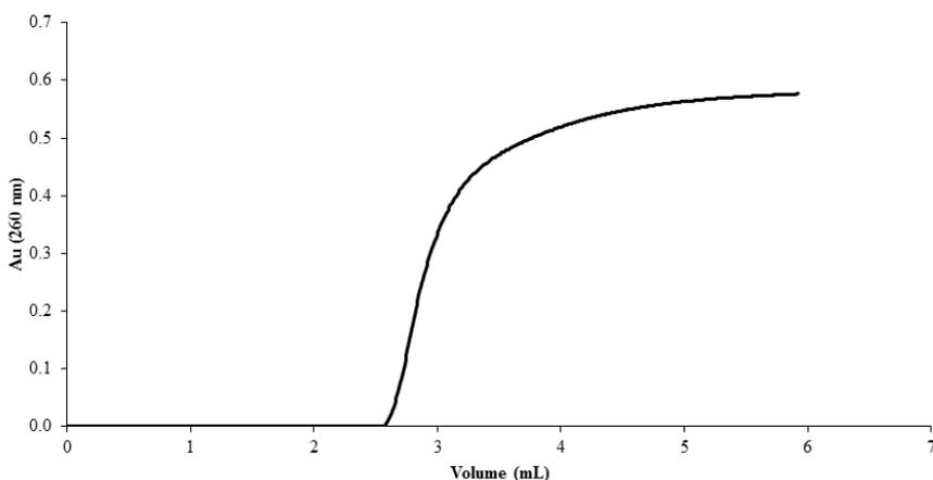
**Figure 3: Plasmid DNA breakthrough curves for the *Capto Adhere* column (2.5 ml) under binding conditions (10 mM Tris-HCl, pH 8.0). The initial pDNA sample was prepared in the running buffer with a final concentration of 0.045  $\mu\text{g/mL}$ . The solution was pumped with a flow-rate of 0.5  $\text{mL}\cdot\text{min}^{-1}$ .**
