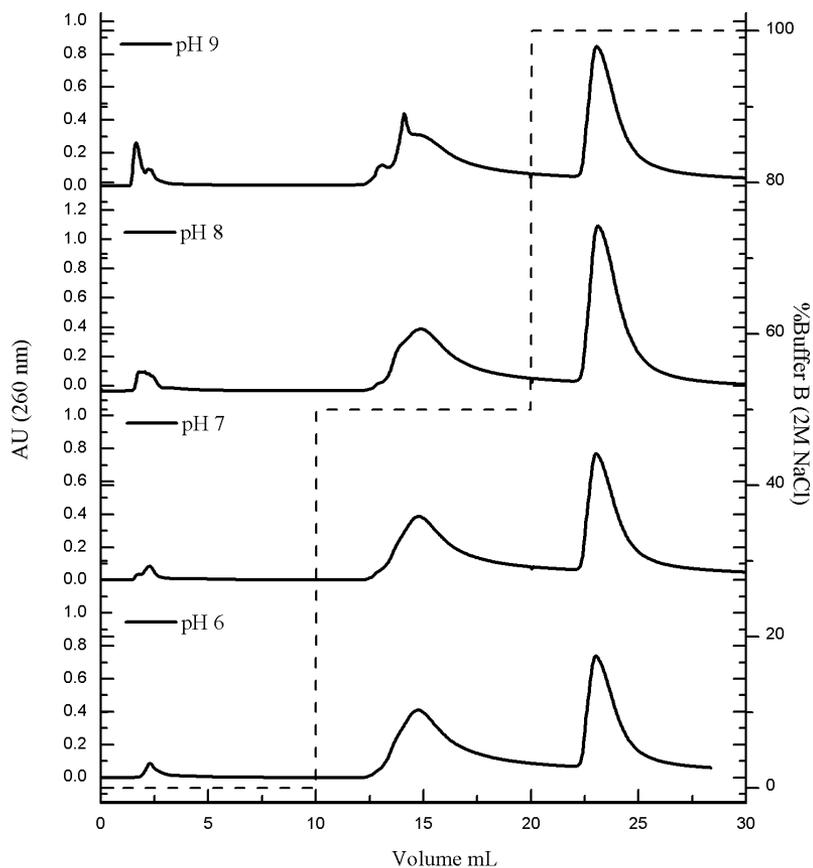
**Figure 4: pH dependency on chromatographic behaviour. In the separation 10 mM Tris-HCl, pH 8.0, was used as running buffer with a flow-rate of 1.0 mL.min<sup>-1</sup>.**
