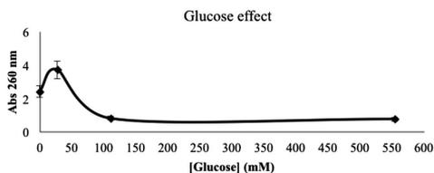
**Fig. 8** Effects of glucose concentration on extraction efficiency of nucleic acids. The process was operated at a constant flow rate of  $0.2 \text{ mL min}^{-1}$  using an applied voltage of 2 V. The results represent an average of three independent measurements.
