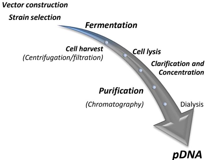
**Figure 3 - Process flow sheet for large-scale purification of plasmid DNA.**
