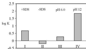
**Fig. 3.** Partitioning of BSA in PEG–polyacrylate two-phase systems. Effect of SDS and pH. All systems contained  $\text{Na}_2\text{SO}_4$  (4 wt%) and BSA (0.2 wt%). Polymer composition as in Table 1 (systems I–IV); pH 5.25 (I, II), pH 6.0 (III), pH 12 (IV). The difference between systems I and II is 0.18 (wt%) SDS in system I.
