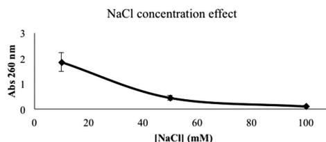
**Fig. 7** Nucleic acid extraction as a function of salt concentration in the lysis process. Salt concentrations used were 10, 50 and 100 mM NaCl. The process was operated at a constant flow rate of 0.2 mL min<sup>-1</sup> using an applied voltage of 2 V. The results represent an average of three independent measurements.
