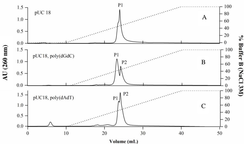
**Figure 4 – Chromatographic behaviour of pDNA (pUC18) in mixtures with smaller dsDNA molecules. A - pUC18 (100µg/mL). B - 1:1 mixture of poly(dGdC) and pUC18; Peak 1 - poly(dGdC) and peak 2 - pUC18; C - 1:1 mixture of poly(dAdT) and pUC18; Peak 1 - poly(dAdT) and peak 2 - pUC18.**
