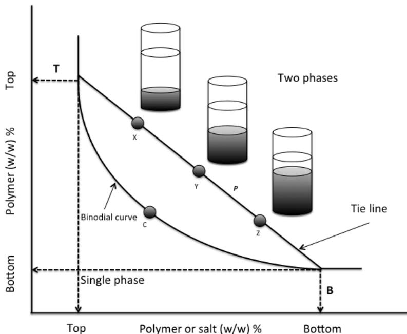
**Figure 8 – A typical phase diagram for polymer-polymer or polymer-salt ATPS. In the figure: C - critical point; T - composition of the top phase; B - composition of the bottom phase; X, Y and Z - total composition of ATPS.**
