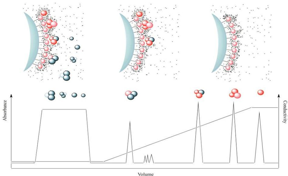
**Figure 10 - Schematic model for AEX chromatography. Elution of the different molecules done by increasing salt concentration (conductivity increases). The elution is achieved in the order that represents the different interactivity between molecules and ligands.**
