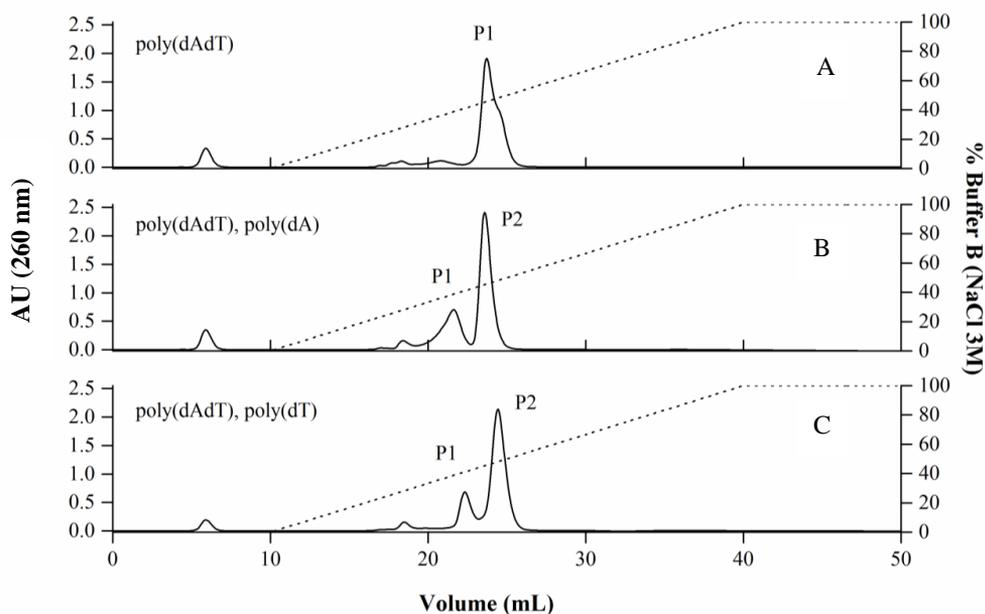
**Figure 3-Chromatographic behaviour of ss and ds DNA molecules on *Capto Q ImpRes*. A - injection of ds poly(dAdT) at a concentration of 100 $\mu$ g/mL; P1, peak 1, represents the dsDNA molecule. B - injection of ds poly(dAdT):poly(dA); P1, peak 1, represents the ssDNA molecule and peak 2 the dsDNA. C- injection of ds poly(dAdT): poly(dT); P1, peak 1, represents the ssDNA molecule and peak 2 the dsDNA.**
