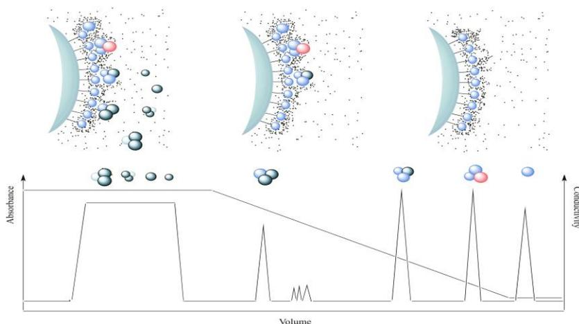
**Figure 12 - Schematic model for HIC. Elution of the different molecules by reducing salt concentration (conductivity decreases) and it is achieved in the order of lower to higher hydrophobicity interaction. Blue represents the hydrophobic groups. Red represents the charged groups. Grey represents the neutral groups.**
