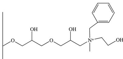
**Fig. 1.** The Capto adhere ligand: N-benzyl-N-methyl ethanolamine. The ligand has a high ion-exchange capacity mixed with hydrophobic moieties, which also promote its stability. The total ionic capacity is 0.09–0.12 mmol Cl<sup>-</sup>/ml and the mean particle size is 75 μm.
