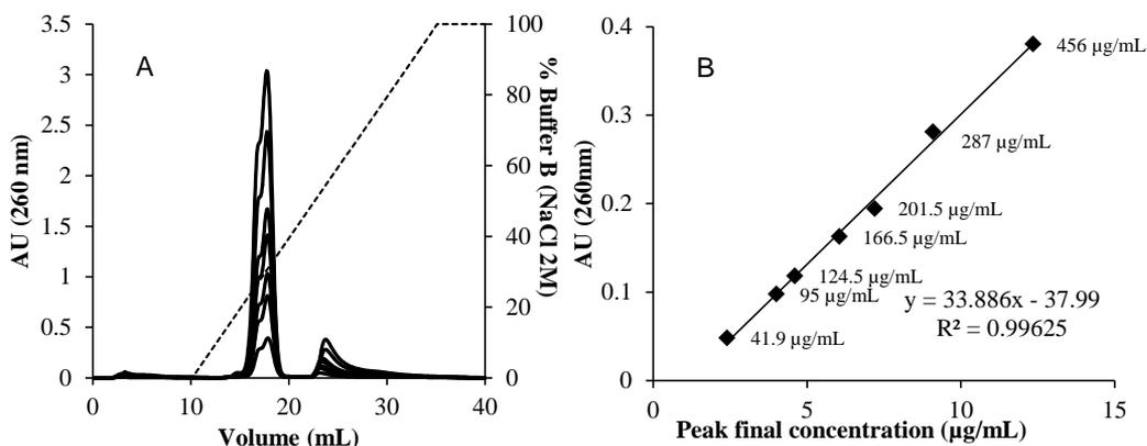
**Figure 6A – Consecutive chromatograms showing different sample concentrations using the same conditions for equilibration and elution [Buffer B is 2.0 M NaCl in Buffer A (10 mM Tris-HCl, pH 8.0)]. Figure 6B – Correlation between concentration of the sample and the peak area corresponding to the pDNA fraction.**
