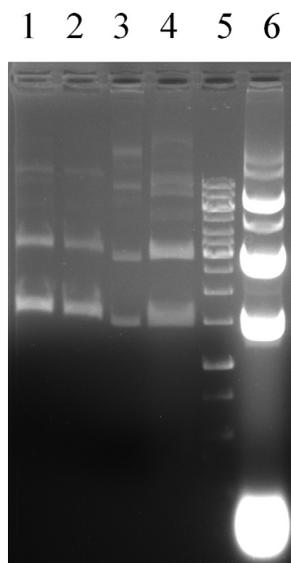
**Fig. 5.** Plasmid DNA analysis in different phases. Lane 1: polyacrylate rich bottom phase of a system with pH 5.4; lane 2: polyacrylate rich bottom phase of a system at pH 5.8; lane 3: salt rich bottom phase from process I; lane 4: salt rich bottom phase from process II; lane 5: Mw-ladder; lane 6: pDNA extracted from *E. coli* by alkaline lysis.
