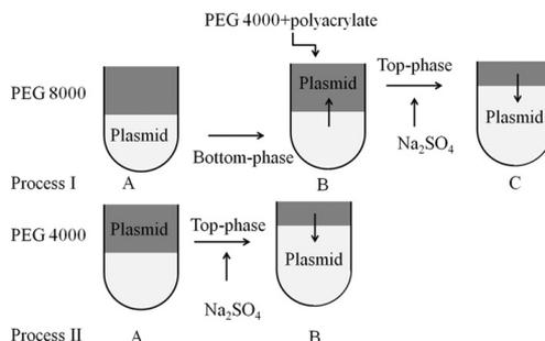
**Fig. 4.** Partitioning of plasmid DNA in PEG/polyacrylate aqueous two-phase systems. In process I pDNA is cross-partitioned between the PAA and PEG phase and then finally back-extracted to a salt phase. In process II the pDNA is back-extracted directly after the primary extraction to the PEG-rich phase. See Section 2.2.7 for composition details.
