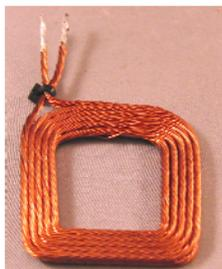
Figure 6: Uncoated coil.
