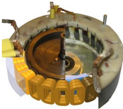
**Figure 1: Superimposed picture of a prototype electrical motor showing the electrical windings (coils) and the surrounding cast SM<sup>2</sup>C-structure. The white material is an additional isolation layer [2].**
