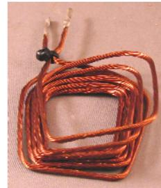
**Figure 8: A coil that has lost its shape.**
