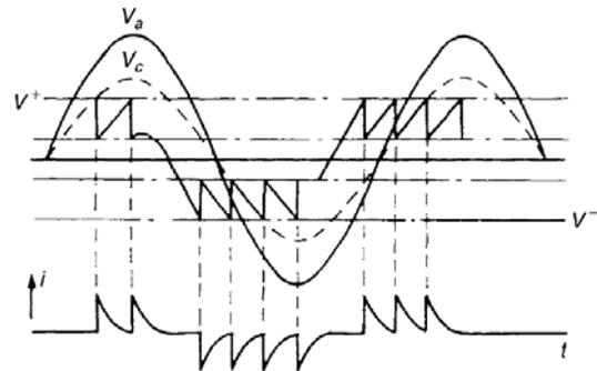
**Figure 5: Sequence of cavity breakdown under alternating voltages [3].**
