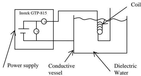
**Figure 9: Schematic view of the electrical test setup.**
