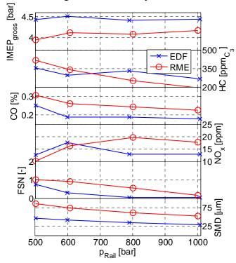
This benefit is reflected in decreasing emissions and increasing IMEP. For the influence of increasing injection pressure on HR, the following is summarised:
