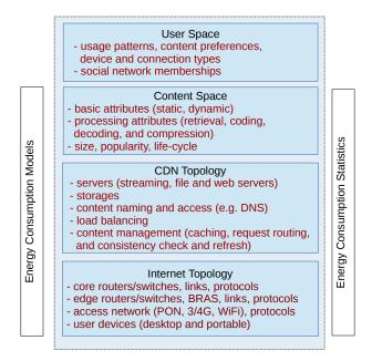
Fig. 1: Building blocks of the proposed simulation package
