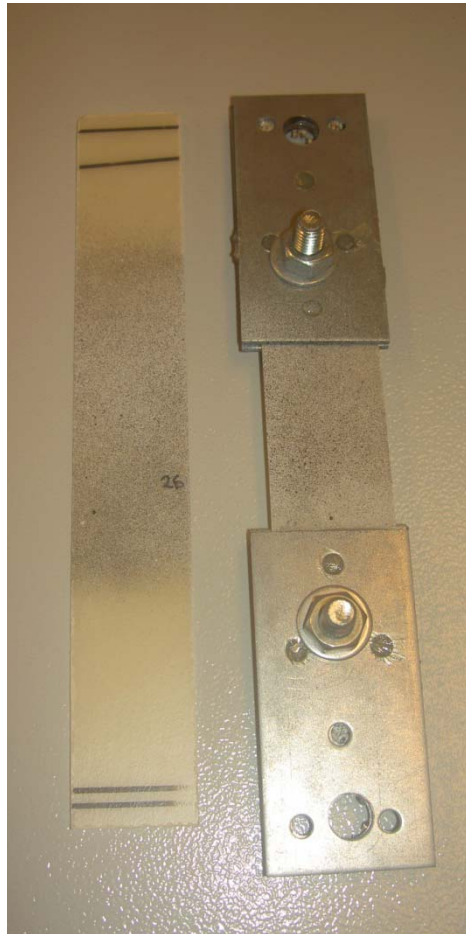
Figure 1. Two specimens, one with aluminium plates glued to the ends.
