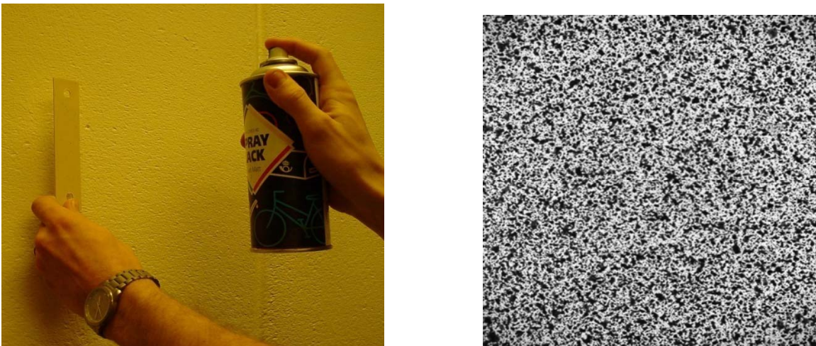
Figure 3. a) Preparation of surface by spraying droplets of black paint. b) Random speckle pattern created by spraying.
