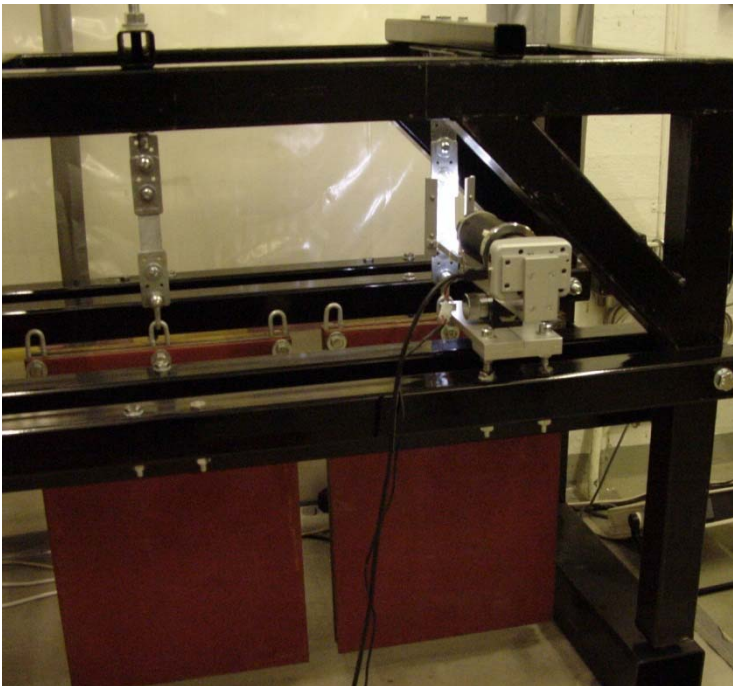
Figure 14. Long time creep tests of several specimens of high pressure laminate simultaneously.
