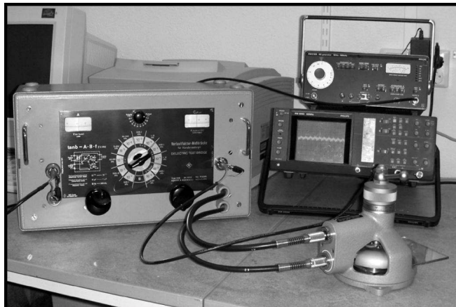
Figure 1: Photograph showing the setup of the parallel plate guard ring capacitor measurement method
