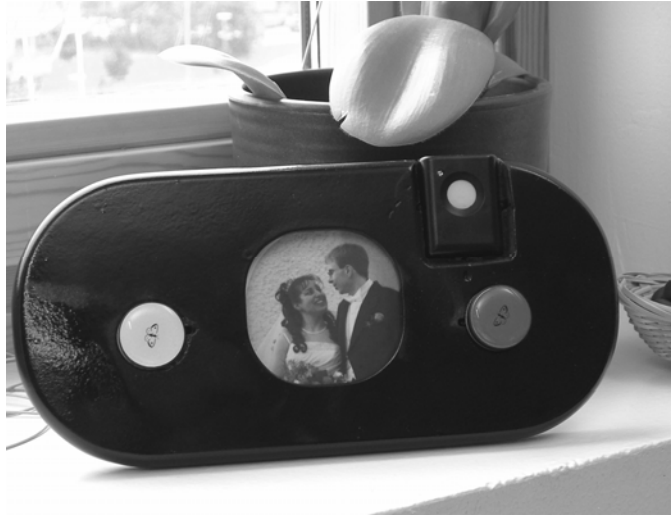
Figure 2. The first working prototype of the photo frame remote control with a small yellow on/off button, and large white and green browsing buttons to the left and right of the photo.
