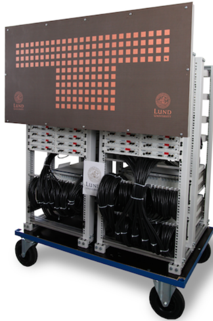
Figure 5.11. The assembled LuMaMi testbed at Lund University, Sweden.
