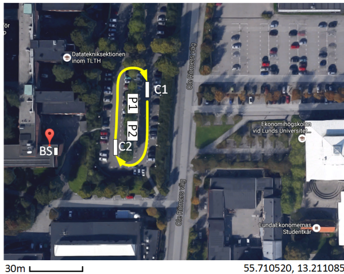
Figure 6.12. Overview of the measurement scenario at the campus of the Faculty of Engineering (LTH), Lund University, Sweden. The BS is placed on the roof with the antenna array facing the parking lot. Arrows indicate the direction of movement for the cars C1 and C2. Pedestrians P1 and P2 moved within the zones indicated by their white boxes.
