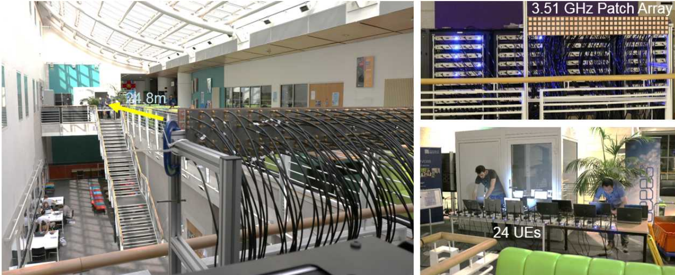
Figure 6.10. Setup to test the maximum number of UEs in a LOS channel. BS and UEs are 24.8 m apart.
