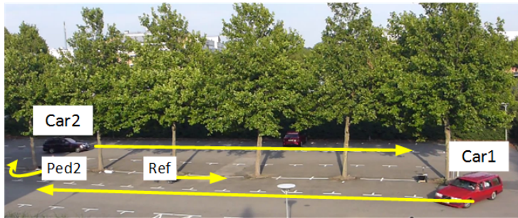
Figure 6.17. 4 second subset of mobility scenario used for temporal analysis. Arrows indicate the movement of each UE over the 4 s duration. Car 2 does not exceed the maximum allowed speed of 29 km/h.
