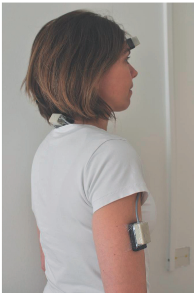
Fig. 2. The placement and size of three of the four pairs of inclinometers including one inclinometer with an integrated data logger (GC-inclinometer) and one validated inclinometer (LT-inclinometer). The black inclinometer is the GC-inclinometer and the white inclinometer with a cable is the LT-inclinometer. The fourth pair is located on the left upper arm.
