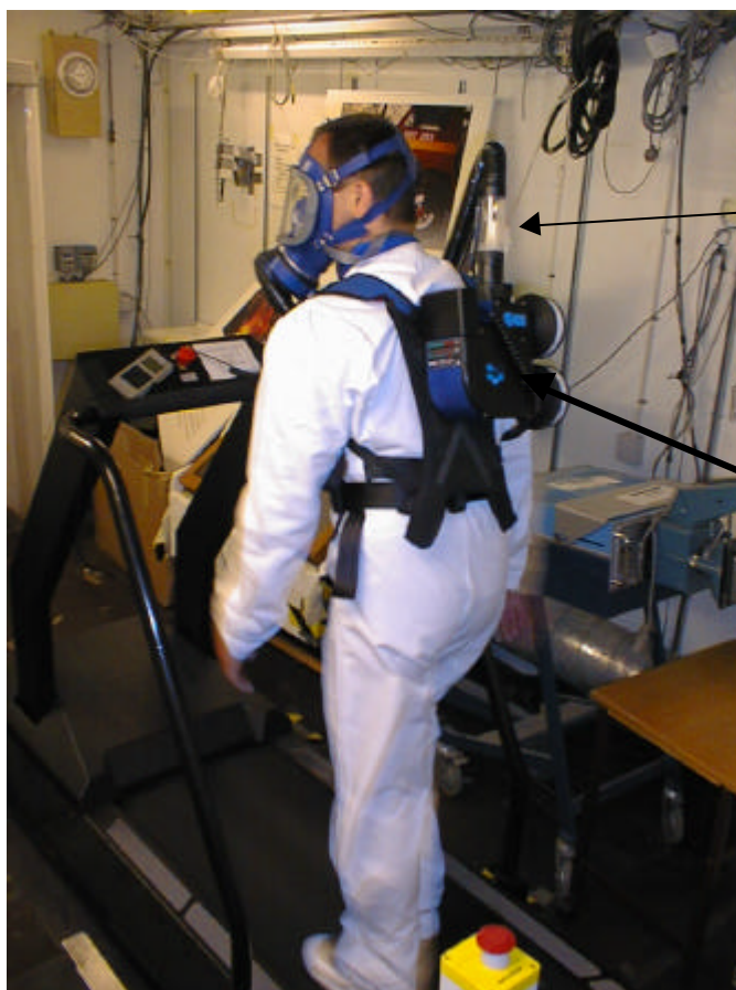
Figure 2. Experimental setup in climatic chamber with treadmill for graded exercise levels. Fan and filter are worn in a separate house on the back. Full face mask is connected to the house via a flexible tube. At the tube end nearest to the house a separate flow meter was mounted.
