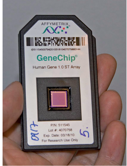
Picture 4. An Affymetrix gene expression microarray. This particular array is the current human chip and contains 28 869 genes. The Lund-zf array, featuring over 22 000 EST sequences corresponding to about 15800 genes, looks just like the chip on the picture. All the gene sequences on an Affymetrix chip are fastened chemically in the small square in the middle of the array. See Box 3 for an explanation of what microarrays do and section 6.4 for description of how the Lund-zf array was designed. The array at the picture has been used in an experiment at the Swegene Centre for Integrative Biology at Lund University (SCIBLU) where all the experiments in this thesis have been hybridized.
