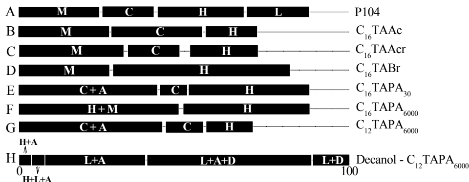
Figure 5 – The scale of the axis goes from 0 to 100 wt% for the respective compound in water. H shows the concentration of decanol. A – water phase, M – micellar, C – micellar cubic, H – hexagonal, L – lamellar and D – decanol.
