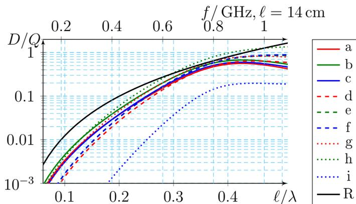
**Figure 8:** Physical bounds on  $D/Q$  for the structures depicted in Fig. 7 obtained using the convex optimization formulation (2.24), [10], when only the antenna region (black in Fig. 7) is optimized. The physical bound on  $D/Q$  for a rectangular PEC surface  $14 \times 7 \text{ cm}^2$ , [11], is depicted in solid black line and labeled “R.”
