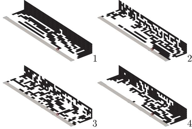
**Figure 4:** GA-optimized structures whose  $Q$ -factors are listed in Table 1. Gray shading—part of the ground plane, black—antenna region part coplanar with the ground plane, bronze—antenna region part normal to the ground plane. Feeding edges are circled.
