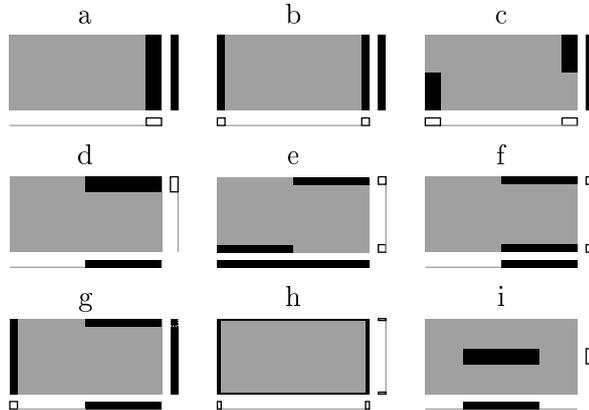
**Figure 7:** Nine simplified wireless-device models limited to a parallelepiped, consisting of a planar ground region extending 90% of one length  $\times$  width face, and an antenna region occupying 10% of the parallelepiped volume. Three side views are depicted for a-g and i, *i.e.*, structures as seen along the length, width and height. A side view along the height and two sections at the symmetry planes are depicted for h. Gray shading—ground plane; black—antenna region, [5, 6].
