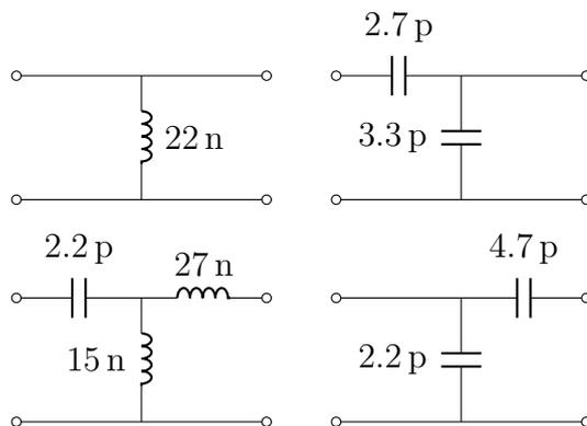
**Figure 6:** Matching networks designed for the structures depicted in Fig. 4 to yield less than  $-6$  dB reflection coefficient magnitude between  $700 \dots 960$  MHz (solid curves in Fig. 5). Component values in SI units. Matching networks numbered as structures in Fig. 4—left to right and top to bottom.
