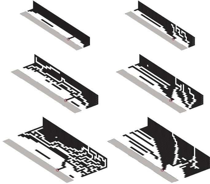
**Figure 3:** Example of genetic algorithm optimized structures (gray shading—part of the ground plane, black—antenna region part coplanar with the ground plane, bronze—antenna region part normal to the ground plane) with  $Q$ -factors depicted in Fig. 2 for  $\ell/\lambda = 0.1$  (left column) and  $\ell/\lambda = 0.5$  (right column), and  $\ell_2 = 0.7$  cm (top row), 1.4 cm (middle row), and 2.8 cm (bottom row). Feeding edges are circled.
