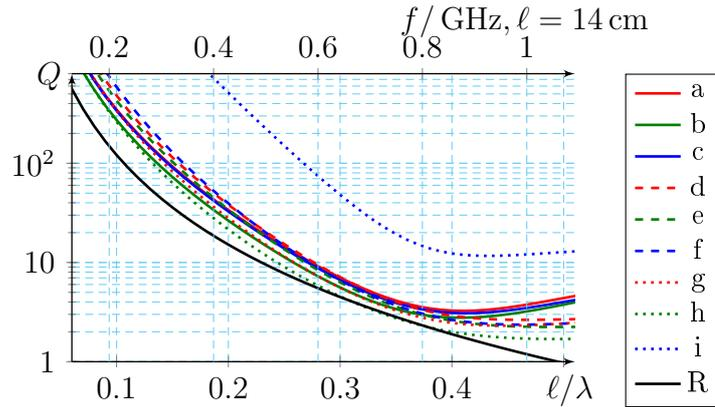
**Figure 9:** The  $Q$ -factors (2.6) achieved by the currents that give the optimum  $D/Q$ -values depicted in Fig. 8. The  $Q$ -factor of a  $14 \times 7 \text{ cm}^2$  PEC rectangle, [11], is labeled “R.”
