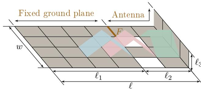
**Figure 1:** Illustration of rectangular mesh element discretization and “rooftop” basis function amplitude for a three-dimensional radiating structure. Metal areas are depicted in gray shading. The amplitudes of three of the total  $7 \times 3 + 6 \times 4 - 4 - 3$  basis functions are depicted in blue, pink and green shading. The feeding edge is marked  $F$ .
