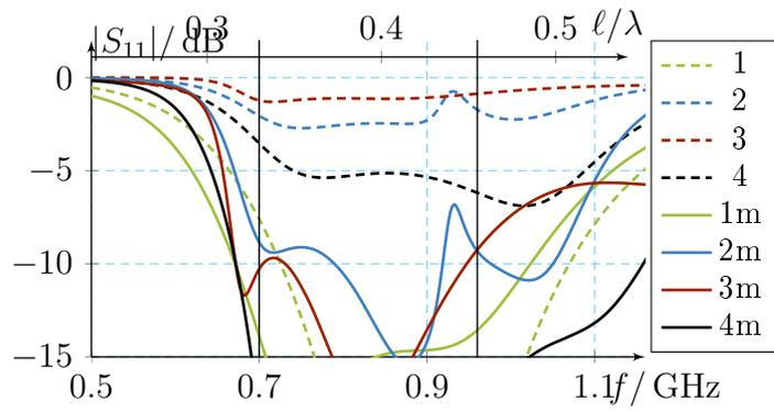
**Figure 5:** Magnitude of  $S_{11}$  at the input of the structures depicted in Fig. 4 without matching network, the curves labeled 1, 2, 3 and 4, and with the matching networks sketched in Fig. 6, the curves labeled 1m, 2m, 3m and 4m.
