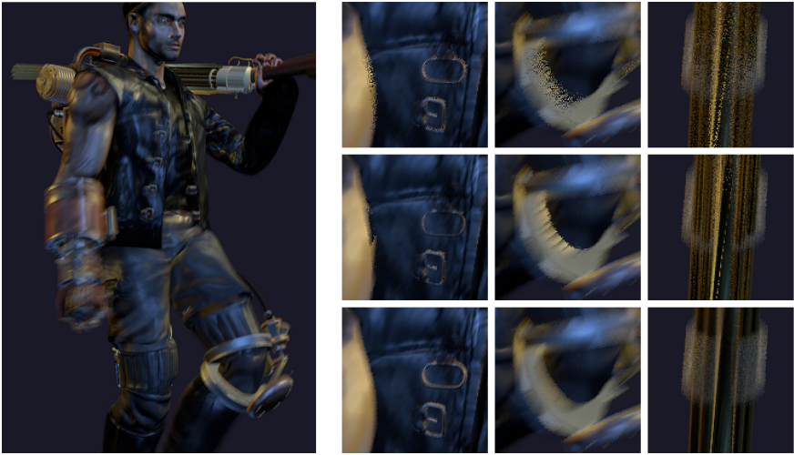
Figure 9: Examples of artifacts caused by writing a single depth compared to correct per-sample depth. The top row uses the depth of the last covered sample, the middle row uses the depth of the nearest sample, and the bottom row uses the correct per-sample depth.
