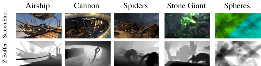
Figure 5: Images from the test scenes used to generate our results. The images are taken from the Heaven benchmark and Stone Giant demo and feature highly tessellated geometry. The Spheres scene is a synthetic benchmark scene intended to stress test highly varying motion. The top row contains reference screenshots without motion (except for the Spheres scene which includes motion), and the bottom row shows depth buffers, rendered using our rasterization framework, including motion blur. All images were rendered at 1920 \times 1080 pixels resolution. The images Airship and Cannon images are courtesy of Unigine Corp., and the Spiders and Stone Giant images are courtesy of BitSquid.
