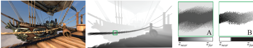
Figure 19: A static scene with a moving camera. The two images to the left show the final rendered image and its corresponding depth buffer, using four samples per pixel. Here, each pixel is displayed using the average depth of its samples. A small crop out of the buffer is shown in inset A. Note the noisy banding resulting from sample coverage in the transition from the rope to the background. Inset B shows the same region, only the gray scale is remapped to only show the pixels where all samples are covered by the rope. Here it becomes apparent that the depth values are irregular due to the samples intersecting the moving rope at different time instances. (Unigine Heaven benchmark courtesy of Unigine Corp.)
