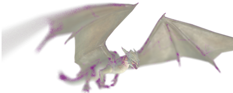
Figure 6: Without conservative rasterization, the regions around triangle edges in the shading texture may have incomplete information, which propagates to the final image as shown here (emphasized in purple color).
