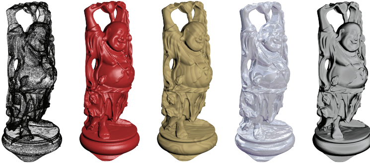
Figure 4: A triangle mesh depicting a laughing Buddha statue with various material properties. The leftmost image shows the finely detailed geometry wire-frame. (Happy Buddha model courtesy of Stanford University Computer Graphics Laboratory)
