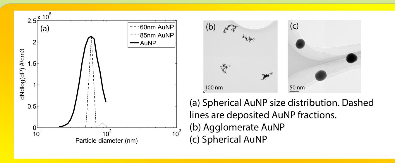
15-16 μg/ml AUNP was selected for deposition into the physiological solutions (a,dashed line). AuNP aersol mass characterisation was performed using an Aerosol Particle Mass Analyzer (3).
