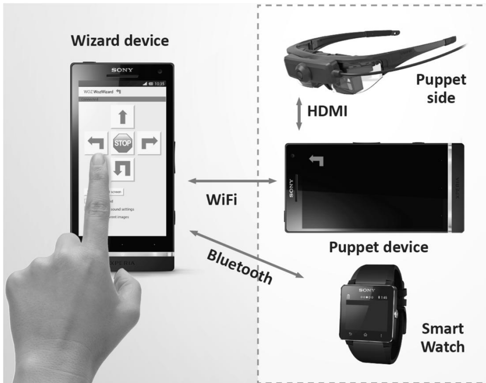
Figure 1. The WozARd architectural setup.
