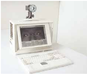
The PowerRefractor is a portable computer with a six-armed retinoscope that measures the refraction of both eyes simultaneously.
