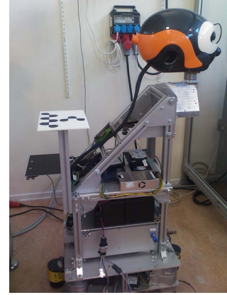
Fig. 1 The mobile robot used for the experiments. The IMU is situated below the black tablet to the left in the picture, and the feature detection pattern used for the vision algorithm is the black and white paper, also to the left in the picture.
