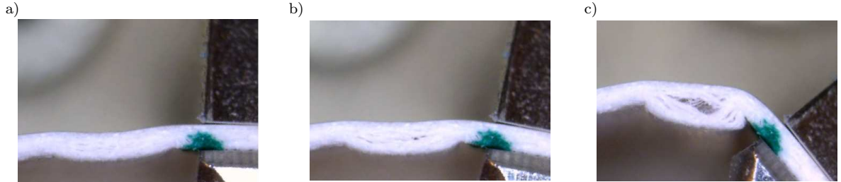
Figure 6: Folding of creased paperboard. The bending angles are approximately (from left to right) 10, 20 and 60 degrees.
