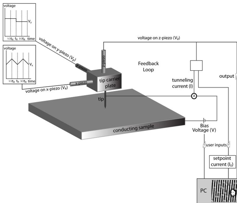
**Figure 2.4** A schematic drawing of the Omicron STM setup. The tip is scanned over the surface with x- and y-piezoelements while the current is kept constant (CCI mode) by a feedback loop which adjusts the movement of the z-piezo. The voltages applied to x- and y- piezoelements are respectively saw tooth and step-like in shape with period of the rastering time ( $t_R$ ).
