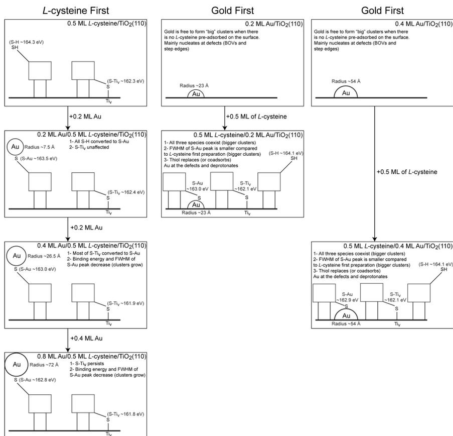
**Figure 4.2.** Schematic representation of the model developed for the co-adsorption mechanism of gold clusters and L-cysteine. The radii of the gold clusters and S 2p<sub>3/2</sub> binding energies are given. Although studied in **Paper 2**, the 0.8 ML gold coverage is not shown.
