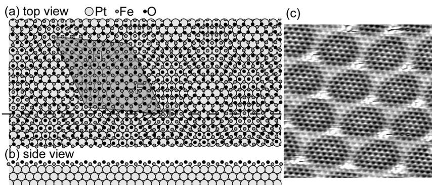
**Figure 3.2** (a) Model of observed structure of FeO(111) thin film on Pt(111) surface as viewed from on top and (b) from the side. Unit cell of moiré pattern is shown as a shaded parallelogram in (a) together with high symmetry domains, T for top, F for fcc, and H for hcp domains. In (c) a  $\sim 10 \times 10\text{ nm}^2$  STM image is shown.
